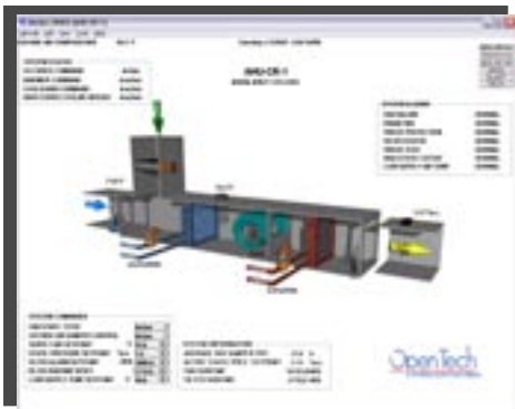
An air handling unit for Lakewood Church: Envision for BACTalk efficiently controls the airflow and air quality inside the megachurch, keeping parishioners cool and free from airborne irritants.
