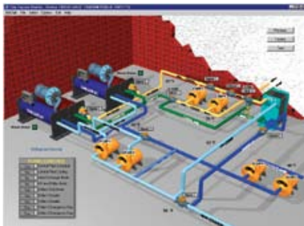
Seamless integration to York chillers at Udall Recreation Center using Alerton BTI global controllers.
